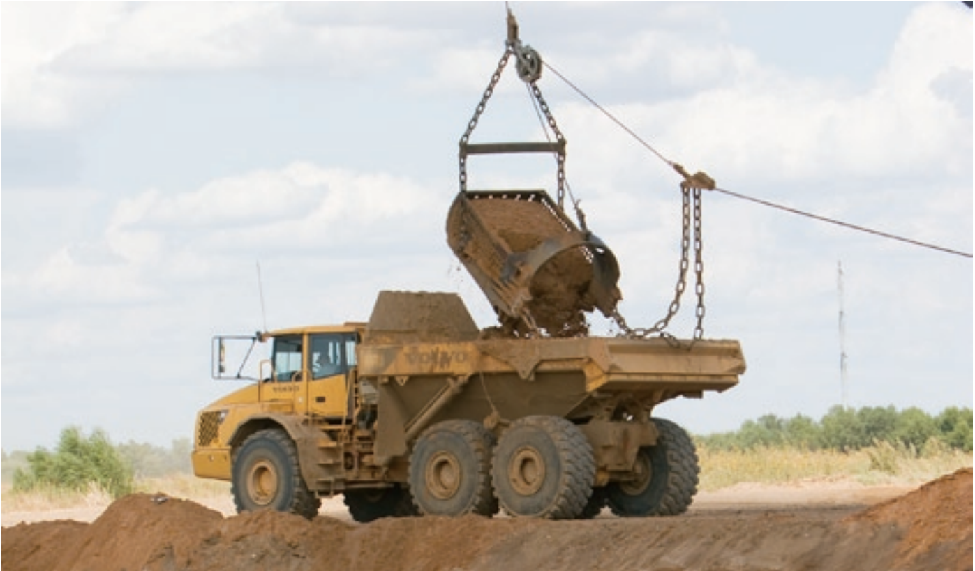
Volvo A40D articulated haulers are the prime movers at the Lattimore Materials sand mine in Ambrose, Texas.
